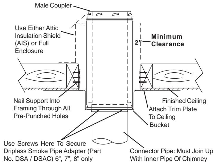
**CAUTION:** Supports Must Be Installed From Below Framing As Shown Here
